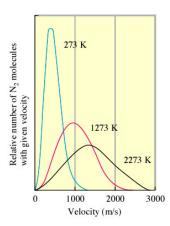
Examine the effect of temperature on the numbers of molecules with a given velocity as it relates to temperature.
