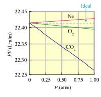
A plot of *PV* versus P for several gases at pressures below 1atm is pictured at left.
