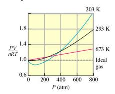
This graph is just for nitrogen gas. Note that although nonideal behavior is evident at each temperature, the deviations are smaller at the higher Ts.
