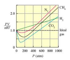
When PV/nRT = 1.0, the gas is ideal All of these are at 200K. Note the P's where the curves cross the dashed line [ideality].
