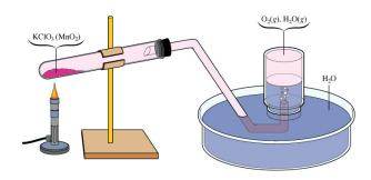
754 torr. The volume of the gas collected was 0.650 L, and the vapor pressure of water at  $22^{\circ}\text{C}$  is 21 torr. Calculate the partial pressure of  $O_2$  in the gas collected and the mass of  $KClO_3$  in the sample that was decomposed.
